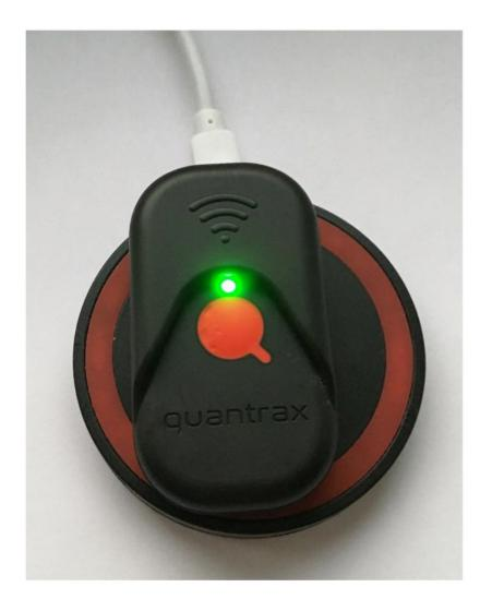
2. First ensure your Quantrax unit is charged and ready to use, To do this place on charger and if light is solid green then leave on charger for Maximum 45 minutes or until green solid light turns off
